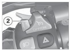
Briefly push button 2 back to return to the speed saved beforehand. Opening the throttle does not deactivate the cruise-control system. If you release the twistgrip the motorcycle will decelerate only to the cruising speed saved in memory, even though you might have intended slowing to a lower speed.
