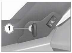
Use the ignition key to unlock seat lock 1 and lift the rear of the seat.
