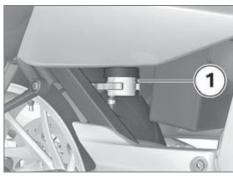
• Check the brake fluid level in rear reservoir 1.
