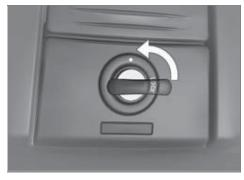
• Turn the key to the in the topcase lock to the position indicated by the dot.
