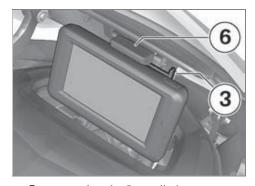
Operate latch 3, pull the navigation device forward out of holder 6 and lift it up and out.
