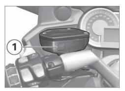
• Check the clutch fluid level in reservoir 1.
