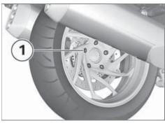
• Fit five bolts 1 and tighten to the specified torque in diagonally opposite sequence.
