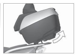
Lift the topcase at the rear and remove it from the luggage carrier.
