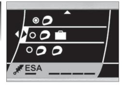
The possible settings for vehicle load appear on the display.
