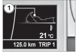
Symbol **1** appears on the display, indicating that the handlebar grip heating is ON.
