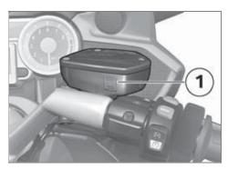
Check the brake fluid level in front reservoir 1.
