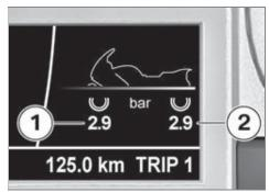
The tyre-pressure readings are based on a reference tyre temperature of 20 °C. The front tyre pressure is on the left 1; the reading on the right 2 is the rear tyre pressure. "---" appears directly after the ignition is switched on, because the sensors do not transmit tyre pressures until the first time the motorcycle accelerates to more than 30 km/h.⊲
