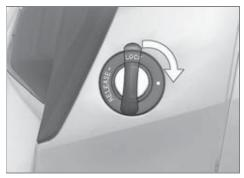
• Turn the key to the in the case lock to the position indicated by the dot.
