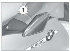
Attempting to adjust the slipstream deflectors while the motorcycle is being ridden can lead to accidents.
