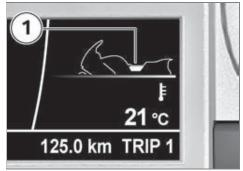
Symbol **1** appears on the display, indicating that the seat heating is ON.
