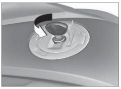
• Use the ignition key to unlock the fuel filler cap and pop the cap open.
