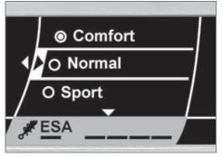
The possible settings for the damping characteristic appear on the display.
