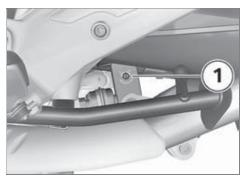
If you want a harder damping characteristic, use the tool from the on-board toolkit to turn ad-
