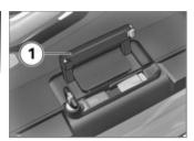
Closing the carry handle while the case lock is in line with the forward direction of travel can result in damage to the locking tongue.
