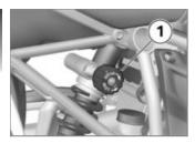
Your motorcycle's handling will suffer if you do not match the spring-preload and damping-characteristic settings. Adjust the damping characteristic to suit spring preload.◀
