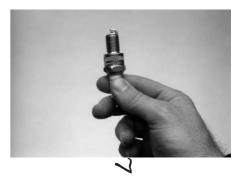
The sparking plug distance should be between 0.6 and 0.7mm.
