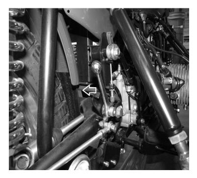
**2wd Engagement Lever** Shifting the lever into the rear locked position will engage 2wd.
