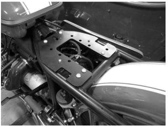
**EFI and Starter Relays** To access the EFI and starter relays you must first remove the seat.
