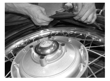
**Step 3** Remove the tube from the tire.
