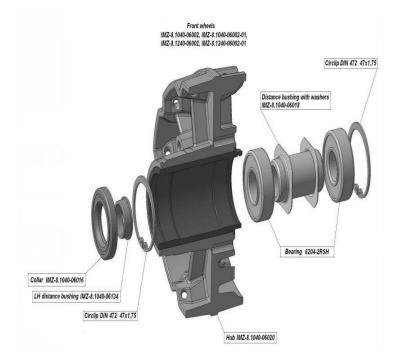
The wheel bearings are sealed type and cannot be service only replaced.
