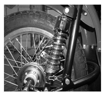
Adjustable Shock Absorbers The shock absorbers have 5 preload adjustments.
