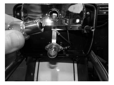
**Step 3** To remove the bulb twist and pull.
