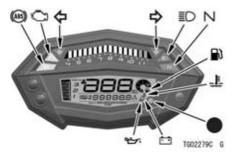
When the ignition switch is turned on, all indicators go on/off as shown in the table. If any indicator does not operate as shown, have it checked by an authorized Kawasaki dealer.
