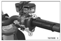
A. Engine Stop Switch B. Starter Button
