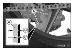
A. Rear Brake Pads B. Lining Thickness
