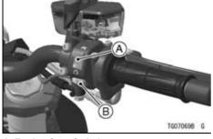
A. Engine Stop Switch B. Starter Button
