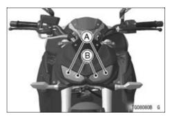
A. High Beams B. Low Beams
