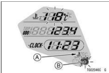
A. Coolant Temperature Warning Symbol B. Red Warning Indicator Light
