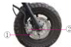
Fig. 32 ① Front brake disc ② Front brake calliper
