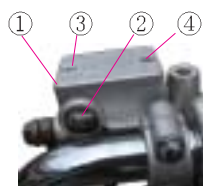
Fig. 30 ① Brake main cylinder ② Sight glass ③ Screw ④ Cover ⑤ Brake calliper
