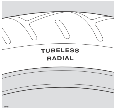
Typical Tyre Marking - Tubeless Tyre
