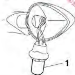
1. Turn signal light bulb
