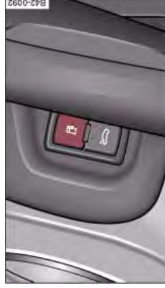
Fig. 112 Tank flap release button in the driver's door trim
