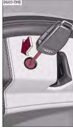
Fig. 39 Locking the door manually
