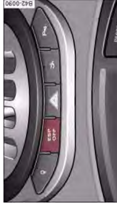
Fig. 110 Centre console with ESP switch
