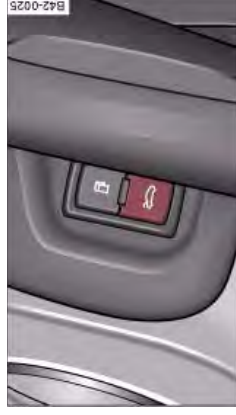
Fig. 40 Driver's door: Unlocking the luggage lid
