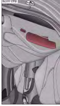
Fig. 99 Location of side airbag in driver's seat
