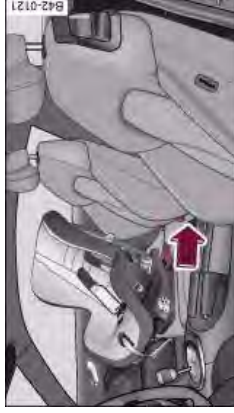
Fig. 109 The ISOFIX child safety seat can be secured after fitting the protective sleeves.
