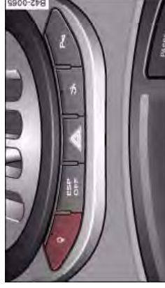
Fig. 76 Centre console: Switch for Audi magnetic ride
