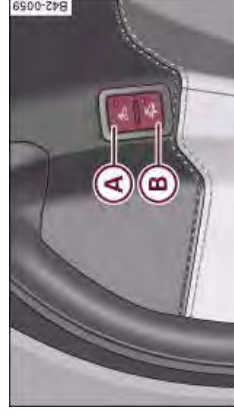
Fig. 43 Switches for the interior monitor in the door trim (only visible when the driver's door is open)
