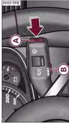
Fig. 8 Windscreen wiper lever: Reset button and rocker switch
