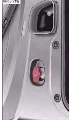
Fig. 121 Luggage compartment: Windscreen washer container
