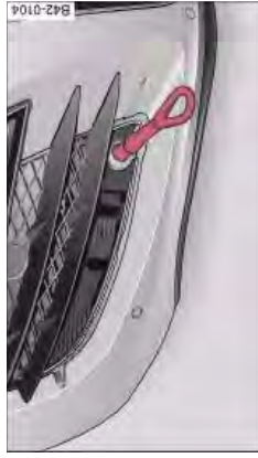
Fig. 132 Detail from front of vehicle, right side with air intake grille removed: Towline anchorage screwed in
