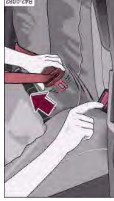
Fig. 94 The latch plate of the belt springs out of the buckle
