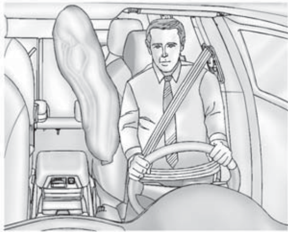
The front center airbag is in the inboard side of the driver seatback.
