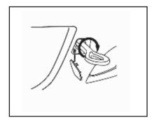
2. Insert the towing hook into the mounting hole and slightly, tighten it clockwise by hand.
