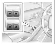
The power windows work when the ignition is in ON/RUN or ACC/ACCESSORY, or in Retained Accessory Power (RAP). Press the switch to open, pull the switch to close. See Retained Accessory Power (RAP) on page 9-27.
