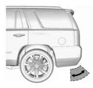
To operate, kick your foot straight up in one swift motion under the center of the rear bumper, then pull it back.
