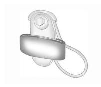
Remove the guide from its storage clip on the interior trim next to the outboard seatback.
