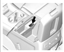
4. Place the new transmitter in the transmitter pocket/insert.
