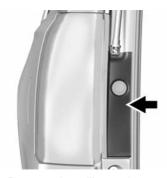
Remove the taillamp closeout cover from the lamp assembly by pulling rearward from the top and bottom at the same time to unfasten the snap tabs.
