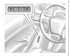
If equipped, the SET, 1, 2, and (Exit) buttons on the driver door are used to manually store and recall memory settings for the driver seat, outside mirrors, power tilt and telescoping steering column (if equipped), and adjustable pedals (if equipped).
