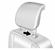
The third row seat head restraint can be lowered for better visibility when the rear seat is unoccupied.
