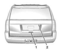
To open the liftgate, press on the power door lock switch or press on the RKE transmitter twice to unlock all doors. Press the touch pad (1) on the underside of the liftgate handle and lift up.
