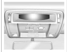
If equipped, push up on the sunglasses bin and release. Push the bin back in halfway to secure the mirror in position.
