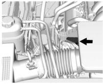
Connect the other end of the negative (-) cable to the metal bracket that is bolted to the engine and supports the resonator, on the vehicle with the dead battery.
