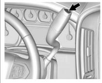
The Tow/Haul Mode adjusts the transmission shift pattern to reduce shift cycling. This provides increased performance, vehicle control, and enhanced transmission and engine cooling when driving down steep hills or mountain grades, towing, or hauling heavy loads.
