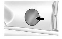
To open the fuel door, push and release the rearward center edge of the door.
