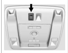
It is recommended that the intrusion and inclination sensors be deactivated if pets are left in the vehicle or the vehicle is being transported. With the vehicle off, press in the front overhead console to turn off the feature.
