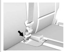
4. Disconnect the rear safety belt mini-latch, using a key in the slot on the mini-buckle, and let the belt retract into the headliner. Stow the mini-latch in the holder in the headliner.
