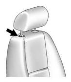
The height of the head restraint can be adjusted. Pull the head restraint up to raise it. Try to move the head restraint to make sure that it is locked in place.
