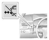
To extend both power assist steps for cleaning, press while the vehicle is in P (Park) or N (Neutral). Press again to retract them. The DIC will display a message.
