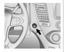
Vehicles with Keyless Access have pushbutton starting.
