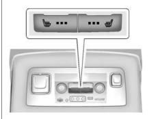
If equipped, the buttons are on the rear of the center console.
