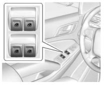
The driver door has switches that control all windows. Each passenger door switch only controls that window. The power windows work when the ignition is in ON/RUN or ACC/ACCESSORY, or in Retained Accessory Power (RAP). See Retained Accessory Power (RAP) on page 9-27.
