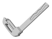
If the vehicle has the Kevless Access system, there is a key in the transmitter.
