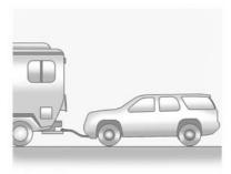
Only dinghy tow four-wheel-drive vehicles with a two-speed transfer case that have an N (Neutral) and a  $4 \downarrow$  setting.
