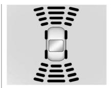
The instrument cluster may have a parking assist display with bars that show "distance to object" and object location information for RPA, and on some vehicles, FPA. As the object gets closer, more bars light up and the bars change color from yellow to amber to red.
