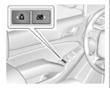
Press to activate the safety locks on the rear doors. The indicator light comes on when activated.
