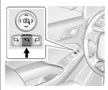
To adjust power folding mirrors, if equipped:
