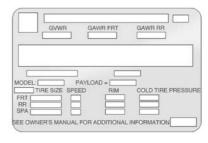
A vehicle specific Certification/ Tire label is attached to the center pillar (B-pillar). The label may shows the size of the vehicle's original tires and the inflation pressures needed to obtain the gross weight capacity of the vehicle. This is called Gross Vehicle Weight Rating (GVWR). The GVWR includes the weight of the vehicle, all occupants, fuel, and cargo.
