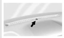
There is a light sensor on top of the instrument panel. Do not cover the sensor, otherwise the headlamps will come on when they are not needed.
