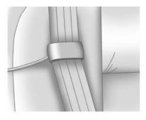
Be sure that the belt is not twisted and it lies flat. The elastic cord must be behind the belt with the plastic guide on the front.
