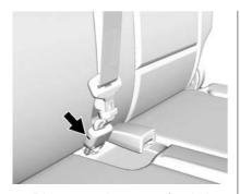
Disconnect the rear safety belt mini-latch using a key in the slot on the mini-buckle, and let the belt retract into the headliner.
