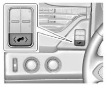
The switch used to adjust the pedals is to the left of the steering wheel.
