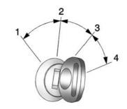
Vehicles with Key Access have an ignition switch with four different positions.
