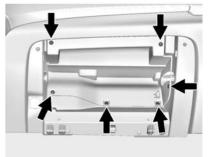
3. Remove the six screws and remove the access plate.
