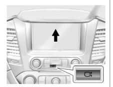
If equipped with storage behind the radio, press and hold  $\bigcirc^{\ddagger}$  to open. There is a USB port inside. See the infotainment manual.
