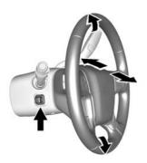
To adjust the power tilt and telescoping steering wheel, if equipped:
