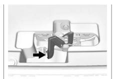
Go to the front of the vehicle to find the secondary hood release. The handle is under the front edge of the hood near the center. Push the handle to the right and at the same time raise the hood. Before closing the hood, be sure all the filler caps are on properly. Then bring the hood from full open to within 15 cm (6 in) from the closed position, pause, and push the front center of the hood with a swift, firm motion to fully close the hood.
