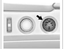
Use the transfer case knob next to the steering wheel to shift into and out of four-wheel drive.
