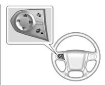
(On/Off): Press to turn the system on or off. A white indicator comes on in the instrument cluster when cruise is turned on.
