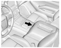
Pull the handle and lift to access the console. There are auxiliary jacks, USB ports, an accessory power outlet, tote compartment, device holder, and SD card reader inside.
