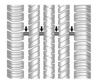
Treadwear indicators are one way to tell when it is time for new tires. Treadwear indicators appear when the tires have only 1.6 mm (1/16 in) or less of tread remaining. Some commercial truck tires may not have treadwear indicators. See *Tire Inspection on page 10-60* and *Tire Rotation on page 10-60* for additional information.
