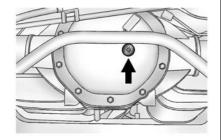
The proper level is 1.0 mm to 19.0 mm (0.04 in to 0.7 in) below the bottom of the fill hole, located on the rear axle. Add only enough fluid to reach the proper level.
