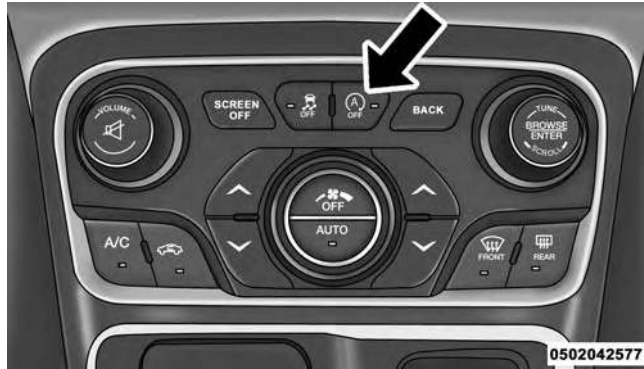
STOP/START OFF Switch
