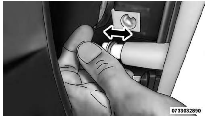
Front Side Marker Lamp Bulb Removal
