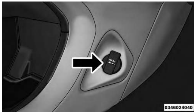
Front Power Outlet
