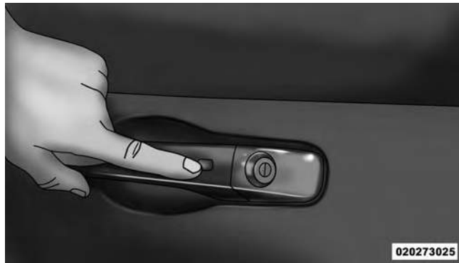
Push The Door Handle Button To Lock
