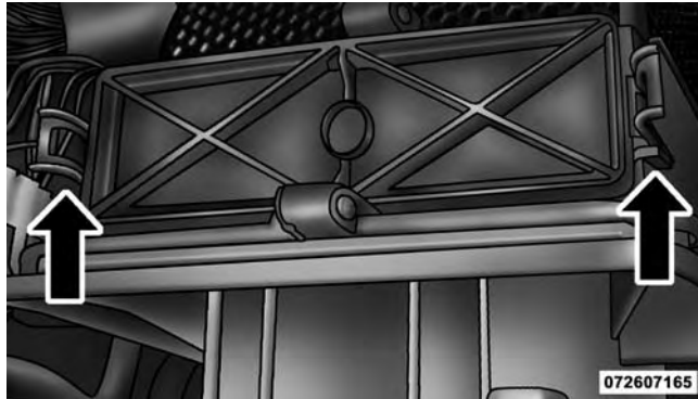
A/C Air Filter Replacement
