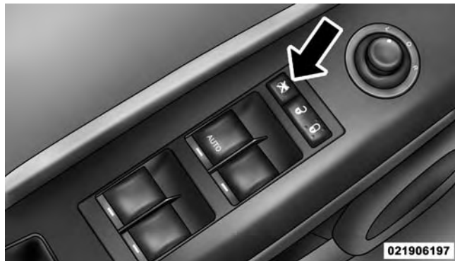
Window Lockout Switch
