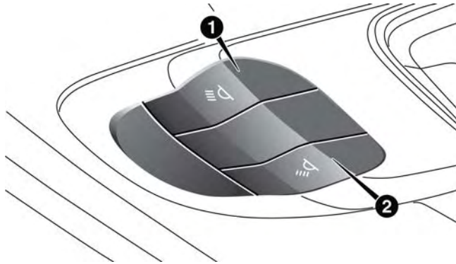
Courtesy Light Switches
