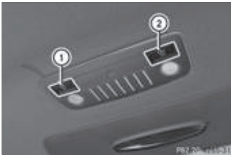
Rear-compartment overhead control panel
