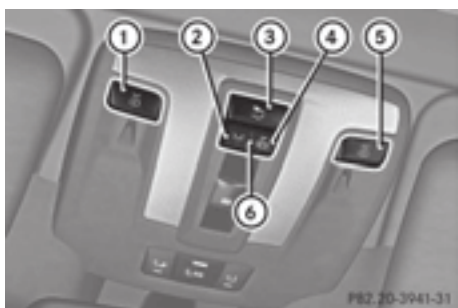
Front overhead control panel
