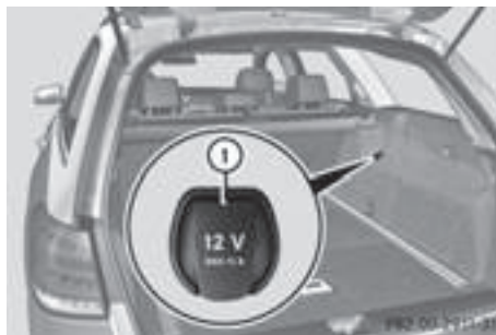
Power socket in the cargo compartment (Wagon)
