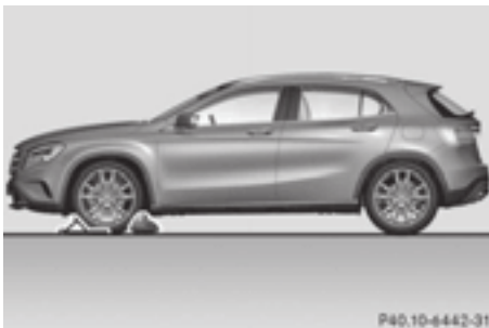
Securing the vehicle on level ground
