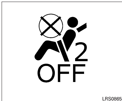
Front passenger air bag and status light
