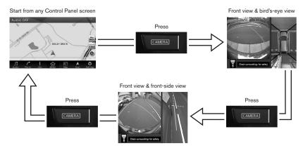
When the shift lever is in the R (REVERSE) position and the CAMERA button 1 is pressed, the following views will display in order:
