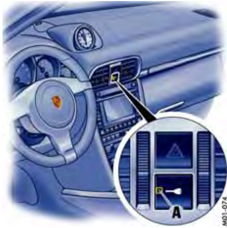
A - Light-emitting diode for alarm system
