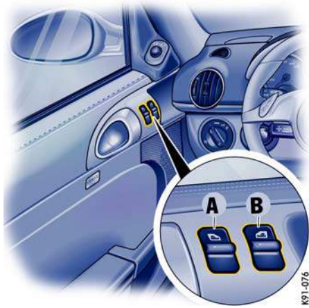
A - Power window in driver's door B - Power window in passenger's door
