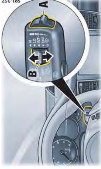
Switches for wiper interval (A) and rear wiper (B)
