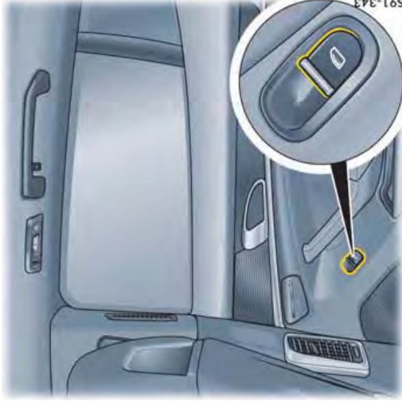
Power window switch in the rear door
