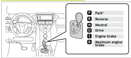
\* The ignition switch must be "ON" and the brake pedal depressed to shift from Park.
