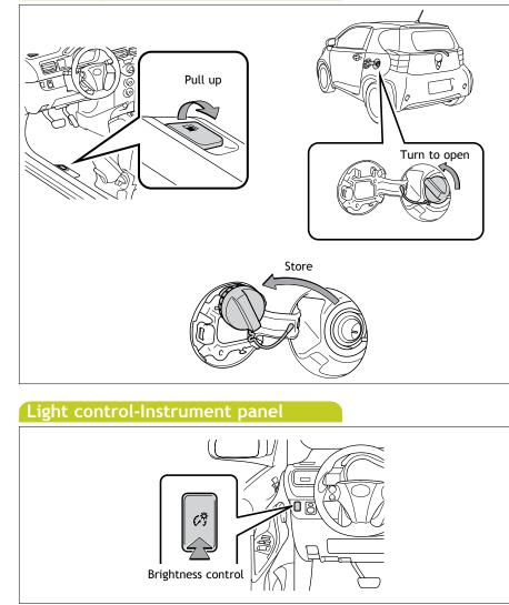
Brightness can be adjusted by pressing the brightness control switch.
