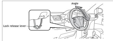
Hold wheel, push lever down, set angle and return lever.
