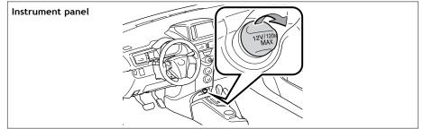
Designed for car accessories. Key must be in the "ACC" or "ON" position to use.
