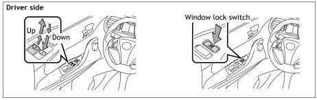
Automatic operation Push the switch completely down or pull it completely up and release to fully open or close. To stop the window partway, operate the switch in the opposite direction.
