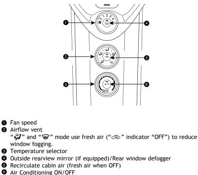
Use fresh air to guickly cool interior, then change to recirculate for cooler air.
