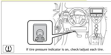
After adjusting tire pressures, or after tires have been rotated or replaced, turn the ignition switch to "ON" and press and hold the ". SET" button until indicator blinks three times. Let the vehicle sit for a few minutes to allow initialization to complete.
