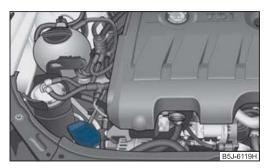
Fig. 147 Engine compartment: Windshield washer fluid reservoir
