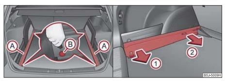
Fig. 64 Luggage compartment: Slacken check points/remove carrier rails
