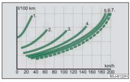
Fig. 134 Fuel consumption in litres/100 km. and speed in km/h.
