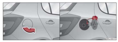
Fig. 11 Right rear side of the vehicle: Fuel filler flap/fuel filler flap with cap unscrewed
