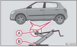
Fig. 156 Changing a wheel: Jacking points for positioning lifting jack
