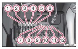
Fig. 168 Schematic representation of fuse assignment at battery
