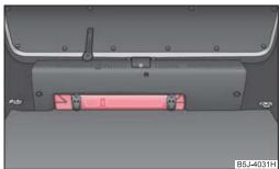
Fig. 150 Placing of the warning triangle
