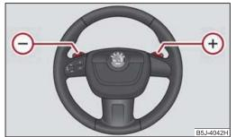
Fig. 103 Multifunction steering wheel: Manual shifting of gears
