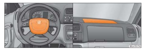
Fig. 115 Driver airbag in the steering wheel/front passenger airbag in the dash panel
