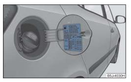
Fig. 148 An opened fuel filler flap with a tyre size and tyre inflation pressure table
