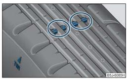
Fig. 149 Tyre tread with wear indicators
