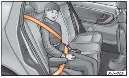
Fig. 128 Child seat in Group 3 installed on the rear seat facing the direction of travel
