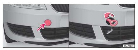
Fig. 161 Front bumper: Cover/installing the towing eye
