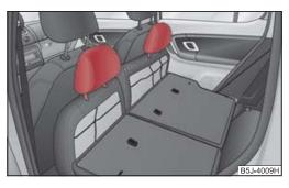
Fig. 55 Rear seats: Inserting head restraints in the seat cushions
