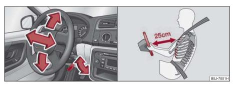
Fig. 94 Adjustable steering wheel: Lever below the steering column/Safe distance to steering wheel
