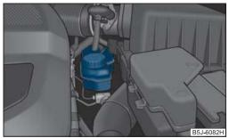
Fig. 144 Engine compartment: Brake fluid reservoir
