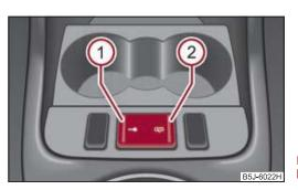
Fig. 26 Centre console: Central locking button
