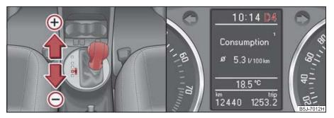
Fig. 102 Selector lever: manual shifting/large information display: Manual shifting of gears
