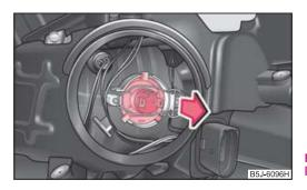
Fig. 170 Removing the light bulb for the low beam and main beam light
