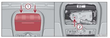
Fig. 34 Detail of the headliner: Points for positioning screwdriver/opening for positioning the key
