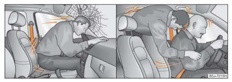
Fig. 111 The driver is catapulted forward if not wearing a belt/The rear seat occupant is catapulted forward if not wearing a belt
