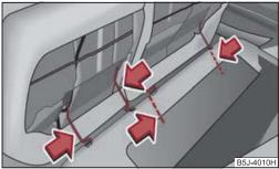
Fig. 56 Removing seat squabs
