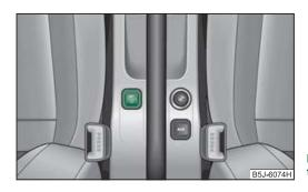
Fig. 132 Button for setting the tyre inflation pressure control value
