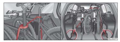
Fig. 72 Securing the bicycles with clamps/securing the bicycles with a strap
