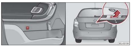
Fig. 28 Unlock the boot lid/handle of the boot lid
