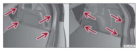
Fig. 57 Luggage compartment: Lashing eyes and fastening elements (Fabia)/(Combi)
