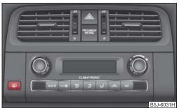
Fig. 43 Switch for rear window heater
