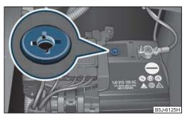
Fig. 146 The battery: Electrolyte level indicator
