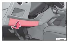
Fig. 163 Bottom side of the dash panel: fuse cover
