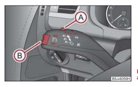
Fig. 99 Operating lever: Rocker button and switch of the cruise control system
