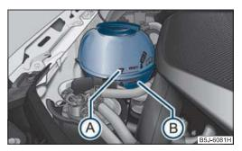
Fig. 143 Engine compartment: Coolant expansion bottle
