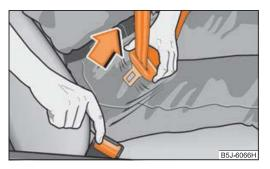
Fig. 114 Releasing lock tongue from belt lock
