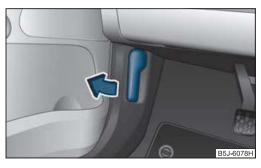
Fig. 139 Release lever engine compartment lid
