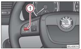
Fig. 108 Multifunction steering wheel: Mobile phone operation The driver can set the basic functions of the telephone by simply operating the buttons located on the steering wheel so that he can concentrate on the traffic situation without being distracted as little as possible by operating the telephone  $\Rightarrow$  fig. 108.
