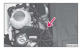
Fig. 160 Jump-starting on vehicles with the START-STOP system
