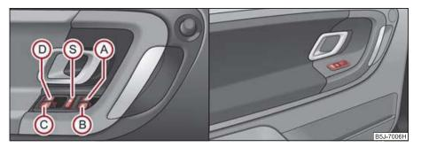
Fig. 32 Buttons on the driver's door/Buttons on the rear doors
