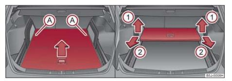
Fig. 63 Luggage compartment: Fold up variable loading floor/remove
