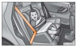
Fig. 126 Child seat with padded table in Group 1 installed on rear seat bench facing the direction of travel
