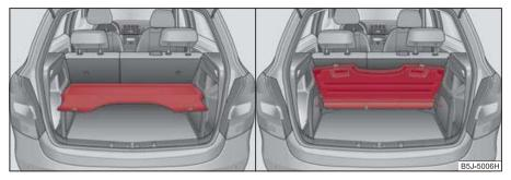
Fig. 61 Luggage compartment cover in the lower position/stowed behind the rear seats
