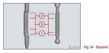
(a) Engine oil **must not** be refilled.
