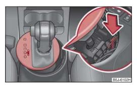
Fig. 104 Selector lever-emergency unlocking
