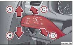
Fig. 8 Turn signal and main beam lever
