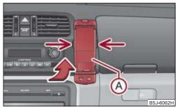
Fig. 106 Universal preparation for the mobile phone
