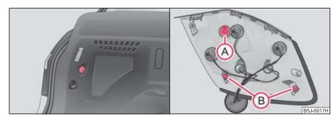
Fig. 177 Remove the rear light unit/install the rear light unit
