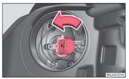
Fig. 172 Removing the light bulb for the main beam light
