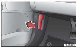
Fig. 12 Release lever engine compartment lid
