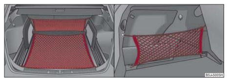
Fig. 58 Fixing net: double horizontal pocket, floor fixing net/double vertical pockets
