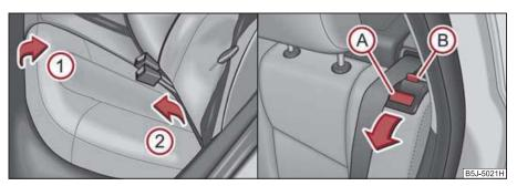
Fig. 54 Fold the seat cushion forwards/unlock the seat backrest
