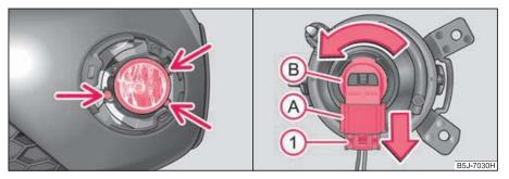
Fig. 175 Front bumper: Fog lights/changing the bulb
