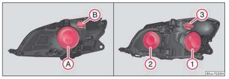
Fig. 169 Fitting position of the bulbs: Halogen headlights/halogen projector headlights
