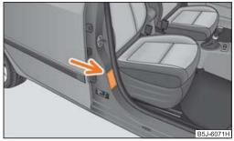
Fig. 123 Sticker on the centre column of the body on the front passenger side.
