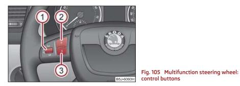
tion system are located on the multifunction steering wheel  $\Rightarrow$  fig. 105. You can of course continue to operate the radio and radio navigation from the unit.
