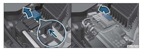
Fig. 145 The battery: Pull up the cover (automatic gearbox)/(manual gearbox)
