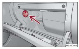
Fig. 81 Storage compartment: Using cooling system
