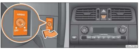
Fig. 122 Switch for the front passenger airbag/indicator light for a switched off front seat passenger airbag
