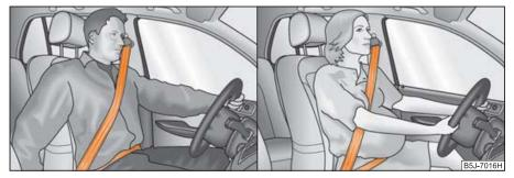
Fig. 112 Routing of belt webbing over the shoulders and the lap belt/Routing of belt webbing for an expectant mother
