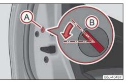
Fig. 27 Emergency locking of the door
