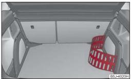
Fig. 89 Flexible storage compartment
