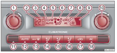
Fig. 93 Climatronic: Control elements
