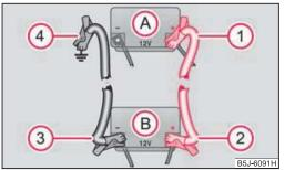
Fig. 159 Jump-starting using the battery from another vehicle: A - flat vehicle battery, B - battery providing current
