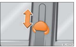
Fig. 113 Front seat: Seat belt height adjuster
