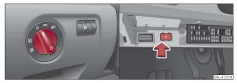
Fig. 35 Dash panel: Light switch/fuse box: Switch for daylight driving lights
