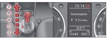
Fig. 101 Selector lever/information display: Selector lever positions
