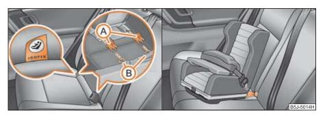
Fig. 129 Locking eyes (ISOFIX system)/Push the ISOFIX child seat into the installed mounting funnels
