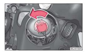
Fig. 171 Removing the light bulb for the low beam and main beam light/low beam light
