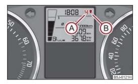
Fig. 17 Shift recommendation for changing gears
