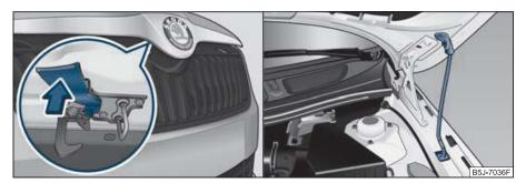
Fig. 140 Radiator grille: Locking lever/securing the bonnet with the bonnet support
