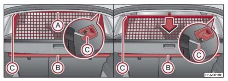
Fig. 66 Pull out the rear bulkhead/roll up
