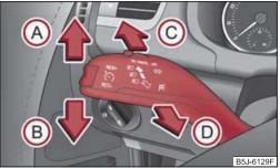
Fig. 39 Turn signal and main beam lever
