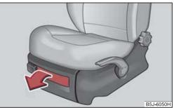
Fig. 85 Front seat: Storage compartment
