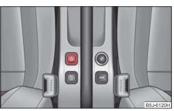
Fig. 100 Centre console: Button for the START-STOP system
