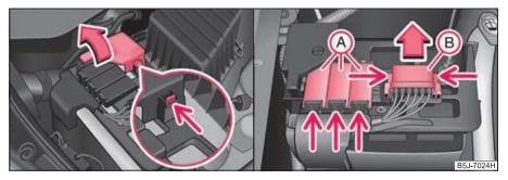
Fig. 167 The battery: Open the positive terminal cover/fuse cover
