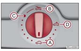
Fig. 33 Detail of the headliner: Control dial for the power sliding/tilting roof
