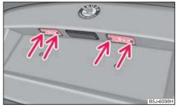
Fig. 176 Remove the licence plate light
