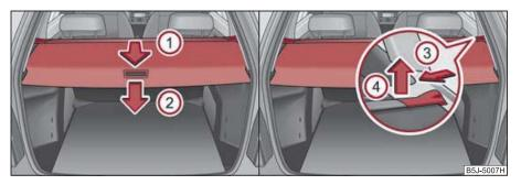
Fig. 62 Luggage compartment: foldable luggage compartment cover/removing foldable luggage compartment cover
