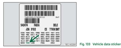
Code **7GG**, **7MB** or **7MG** on the vehicle data sticker, see  $\Rightarrow$  fig. 133, indicates that your vehicle is equipped with a diesel particle filter. The vehicle data sticker is located on the floor of the luggage compartment and is also stated in the Service schedule.
