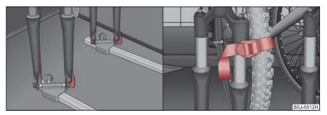
Fig. 71 Put in the bicycle/fastening the front wheel
