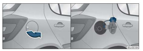
Fig. 138 Right rear side of the vehicle: Fuel filler flap/fuel filler flap with cap unscrewed
