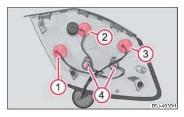
Fig. 178 Rear light unit: Fitting position of the bulbs
