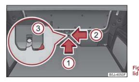
Fig. 29 Emergency unlocking of the boot
