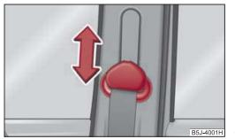
Fig. 4 Front seat: Seat belt height adjuster
