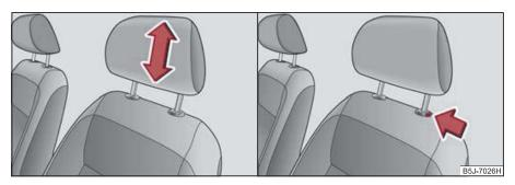
Fig. 52 Head restraint: Adjusting/pulling out
