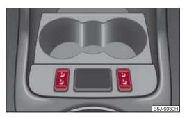
Fig. 53 Rocker switch: Front seat heating
