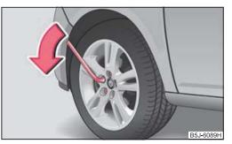
Fig. 155 Changing a wheel: Slackening wheel bolts
