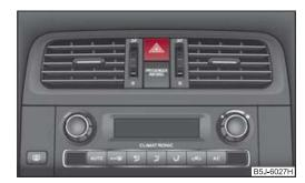
Fig. 38 Dash panel: Switch for hazard warning lights
