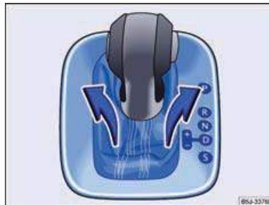
Fig. 103 Remove the cover of the shift gate.
