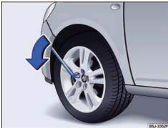
Fig. 109 Changing a wheel: Slackening the wheel bolts.
