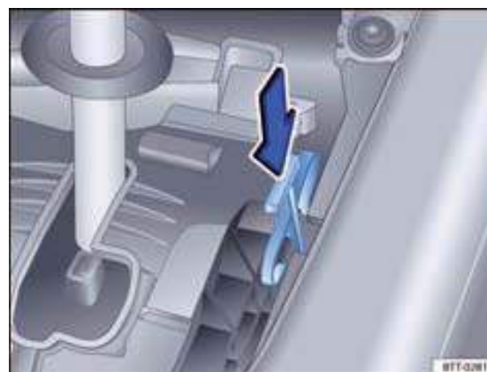
Fig. 104 Emergency unlock the release lever lock.
