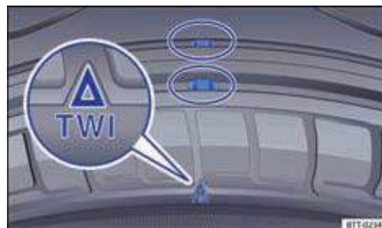
Fig. 94 Tread: Wear indicator.
