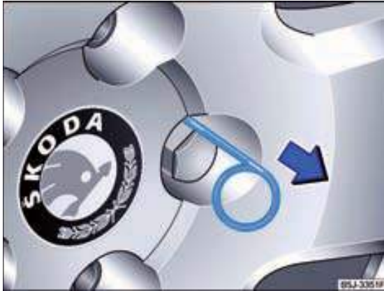
Fig. 108 Pulling off the caps from the wheel bolts.
