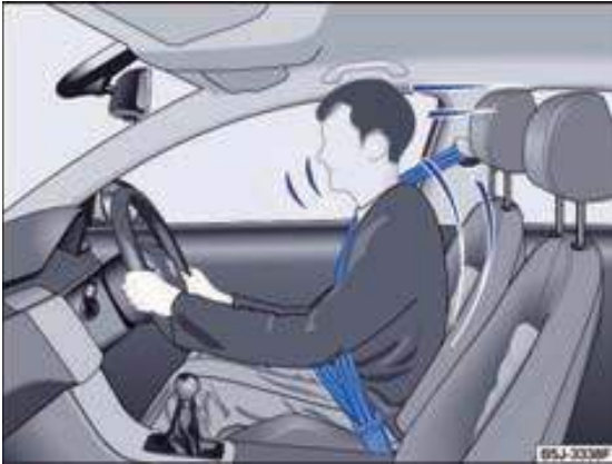
Fig. 35 Driver wearing a seat belt who is caught by the correctly fastened and adjusted seat belt in a sudden braking manoeuvre.
