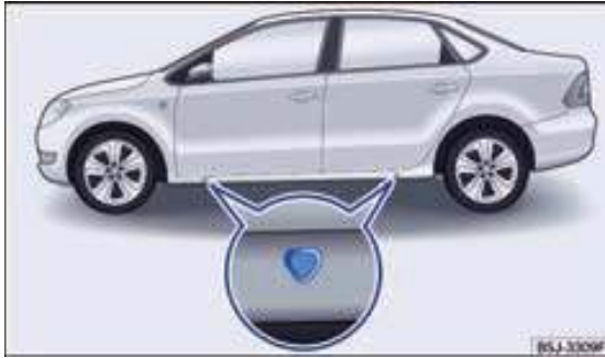
Fig. 111 Jacking points for positioning the jack.
