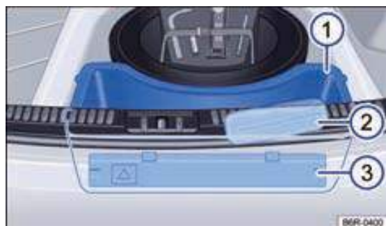
Fig. 100 In the boot: Storage compartment for the warning triangle.
