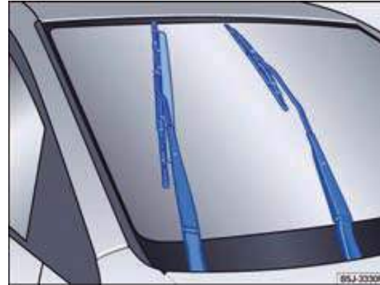
Fig. 89 Windscreen wiper in service position.
