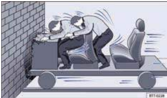
Fig. 32 A vehicle hits the wall with occupants not wearing seat belts.
