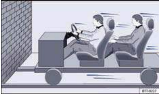
Fig. 31 A vehicle moves towards a wall with occupants not wearing seat belts.
