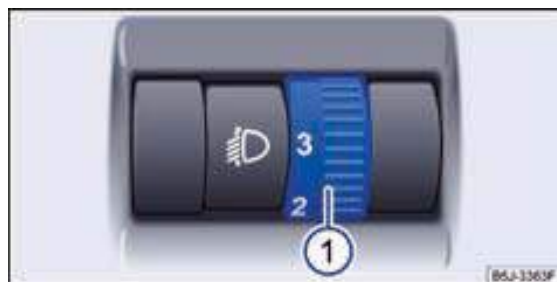
Fig. 46 Beside the steering wheel: Control for headlight beam adjustment ①.
