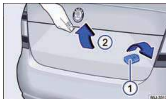
Fig. 20 Opening the boot lid from the outside.
