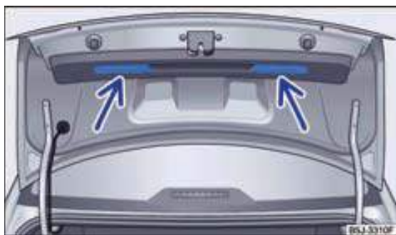
Fig. 21 Open boot lid: Recesses for closing.
