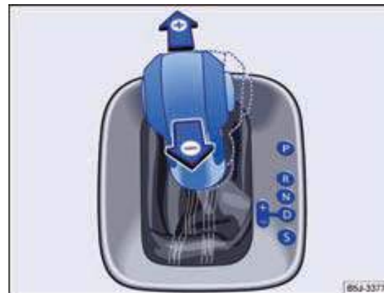
Fig. 71 Selector lever in Tiptronic position.
