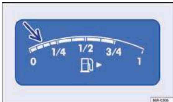
Fig. 79 In the instrument cluster: Fuel gauge for petrol and diesel fuel.
