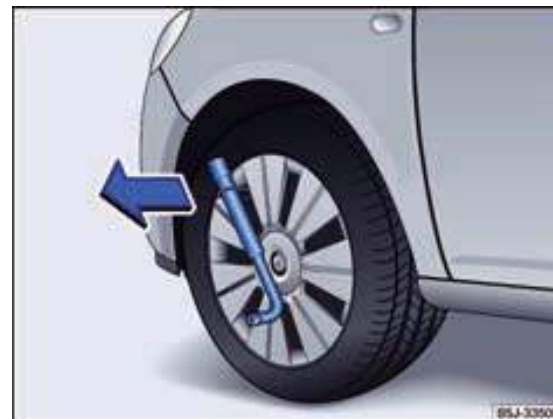
Fig. 107 Removing a push-on type wheel trim.
