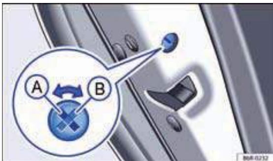
Fig. 17 In the rear left door: Child safety lock (A) is on, (B) is off.
