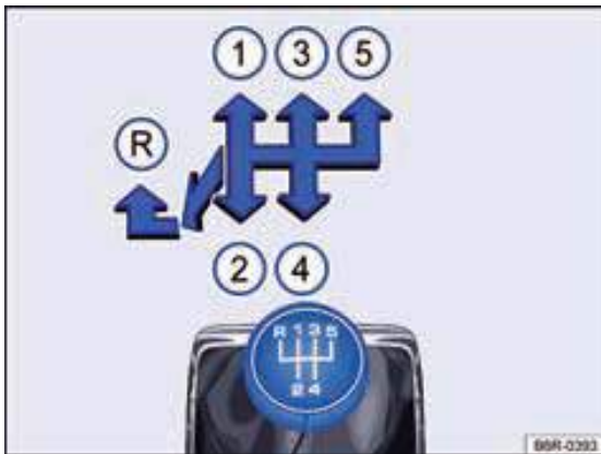
Fig. 69 Shift pattern of the 5-speed manual gearbox.
