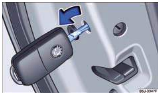
Fig. 102 Emergency locking the vehicle with the vehicle key (the emergency lock is covered by a rubber seal).
