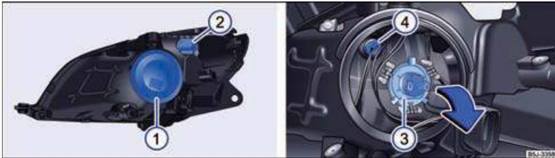
Fig. 118 Rear view of the right H4 headlamp.
