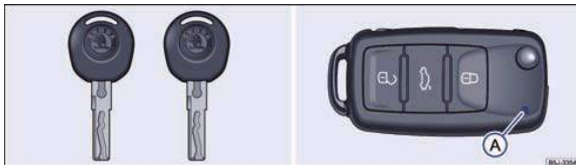
Fig. 15 Key without remote control / remote control key
