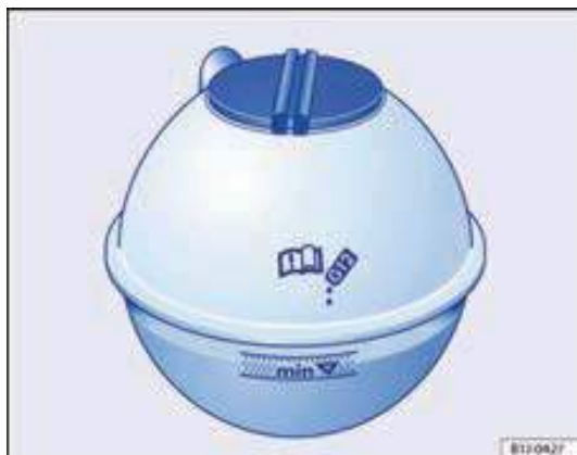
Fig. 86 In the engine compartment: Marking on the engine coolant expansion reservoir.
