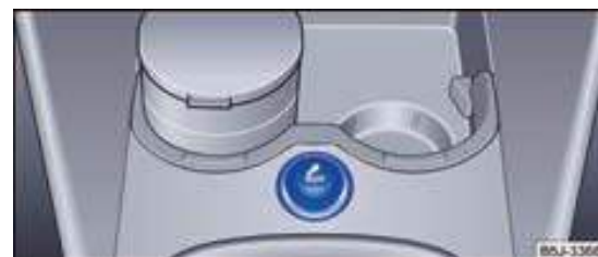
Fig. 65 Front centre console: 12-Volt power socket.
