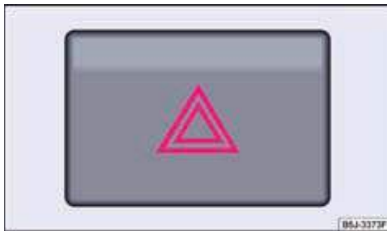
Fig. 99 In the centre of the instrument panel: Switch for the hazard warning light system.
