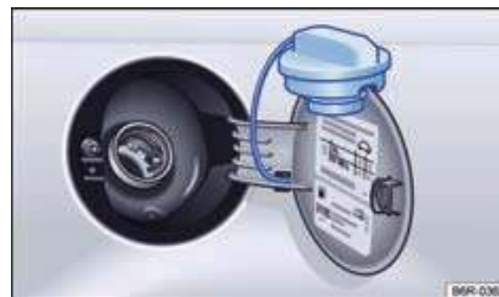
Fig. 81 Open fuel filler flap with attached fuel filler cap.
