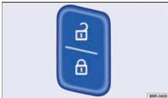
Fig. 16 In the driver's door: Central locking button.
