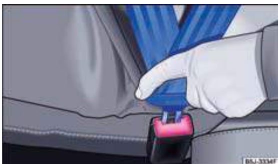
Fig. 36 Insert the lock tongue of the seat belt into the belt buckle.
