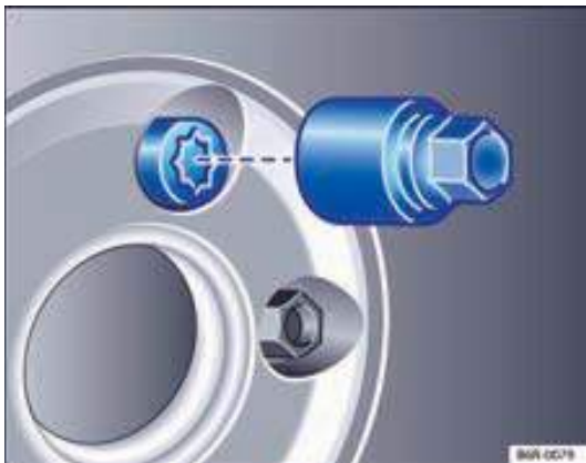
Fig. 110 Changing a wheel: Anti-theft wheel bolt and adapter.
