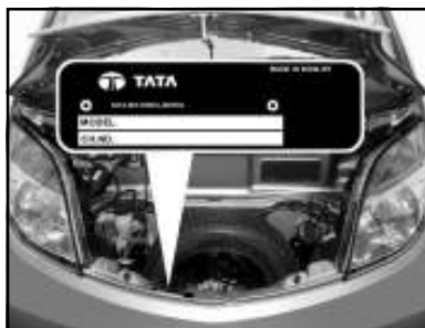
Chassis Number Plate on Fire Compartment
