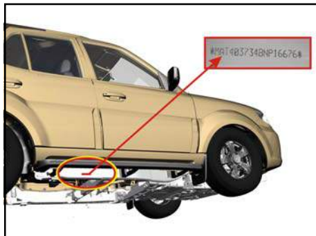
Chassis No. - Punched on RH Long member
