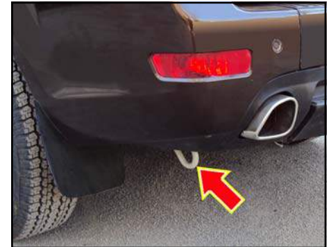
Tow Hook Attachment Location at Rear
