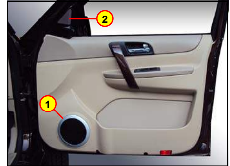
1. Speaker on front door trim 2. Tweeter in the inner cover of ORVM
