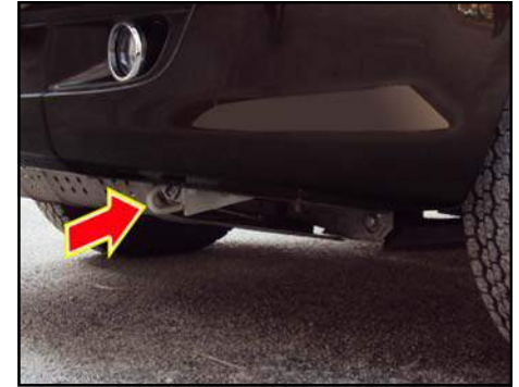
Tow Hook Attachment Location at Front
