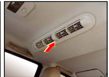
A.C. air vents on roof for Second and Third row seats
