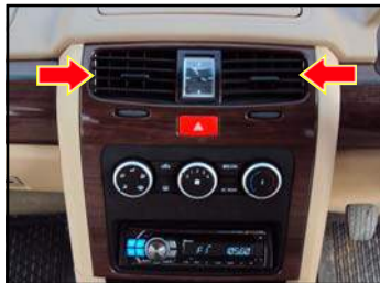
A.C. air vents on central Console for front seat
