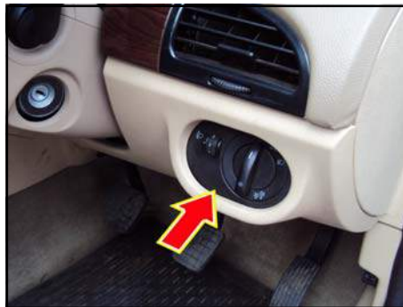
Location of master light switch
