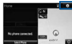
STEP 6 On your Toyota Vehicle Entune Multimedia Head Unit, Select SETUP BUTTON on the Home Screen.
