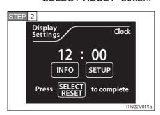
Press the "INFO" button to adjust the hours and the "SETUP" button to adjust the minutes.
