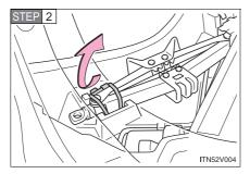
Unlock the tightening strap.
