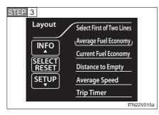
When a 2-line layout is selected in STEP 2, the "Layout" screen is displayed. First, using the "INFO" and "SETUP" buttons, select the item you wish to display in the first line, and then press the "SELECT RESET" button.
