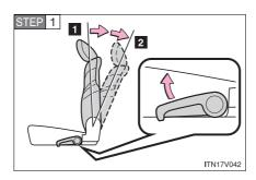
Fold the seatback while pulling the lever. Return the seatback and secure it as upright as possible (1st lock position). Adjust the seatback to the 3rd lock position.  $(\rightarrow P. 70)$
