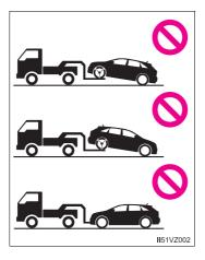
Be sure to transport the vehicle with all four wheels raised off the ground. If the vehicle is towed with the tires contacting the ground, the drivetrain or related parts may be damaged, the vehicle may fly off the truck.
