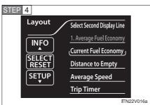
Using the "INFO" and "SETUP" buttons, select the item you wish to display in the second line, and then press the "SELECT RESET" button.
