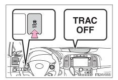
To turn the TRAC system off, quickly press and release
