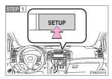
Press the "SETUP" button while the vehicle is stopped.
