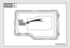
Remove the fuse with the pullout tool.
