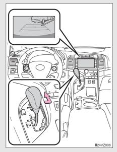
Vehicles with smart key system: The rear view image is displayed when the shift lever is in "R" and the "ENGINE START STOP" switch is in IGNITION ON mode.
