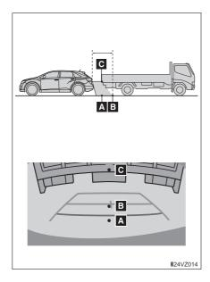
Visually check the surroundings and the area behind the vehicle. On the screen, it appears that a truck is parking at point B. However, in reality if you back up to point A, you will hit the truck. On the screen, it appears that A is closest and C is furthest away. However, in reality, the distance to A and C is the same, and B is farther than A and C.
