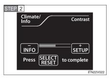
Press the "INFO" or "SETUP" button to adjust the contrast.
