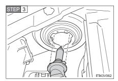
Replace the light bulb, and install the light bulb.
