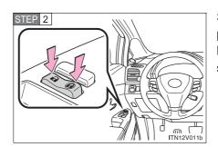
Shift the shift lever to "P" or "N", press and hold the driver's door lock switch ( or ) for about 5 seconds then release.
