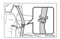
Pass the outer seat belts and plates through the seat belt hangers to prevent the shoulder belts from being damaged.
