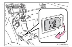
Open the cover and connect an iPod using an iPod cable.
