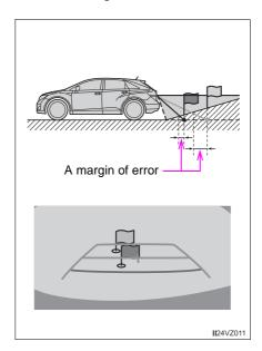
The distance guide lines will appear to be closer to the vehicle than the actual distance. Because of this, objects will appear to be farther away than they actually are. In the same way, there will be a margin of error between the guide lines and the actual distance/course on the road.
