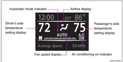
The settings display will differ according to the situation. If pressed while in automatic mode, the status of all settings will be displayed for a number of seconds.
