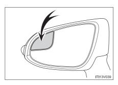
The Blind Spot Mirrors increase the view of surrounding area to assist the driver when checking surrounding area before changing lanes.
