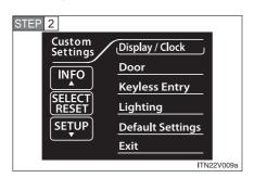
Select "Display / Clock" by pressing the "INFO" or "SETUP" button, and press the "SELECT RESET" button.
