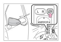
Press the switch to fold the mirrors.
