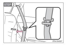
Pass the outer seat belts and plates through the seat belt hangers.
