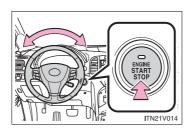
The green indicator light on the "ENGINE START STOP" switch will flash and a message will be shown on the multi-information display (TFT type only). To free it, press the "ENGINE START STOP" switch while turning the steering wheel slightly in either direction.
