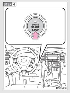
Press the "ENGINE START STOP" switch.
