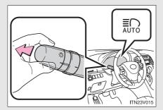
Push the lever away from you with the headlight switch in AUTO position when the "ENGINE START STOP" switch is in IGNITION ON mode (vehicles with smart key system) or the engine switch is in the "ON" position (vehicles without smart key system).
