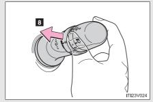
Wash/wipe operation Wipers operate automatically.
