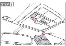
Press and hold one of the HomeLink® buttons and the transmitter button. When the HomeLink® indicator light changes from a slow to a rapid flash within 20 seconds, you can release both buttons.
