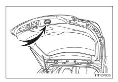
Lower the back door using the back door handle, and make sure to push the back door down from the outside to close it.
