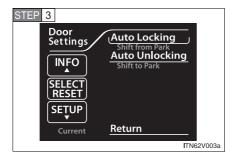
Select the setting you wish to change by pressing the "INFO" or "SETUP" button, and press the "SELECT RESET" button.
