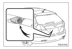
The camera for the rear view monitor system is located above the license plate.
