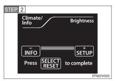
Press the "INFO" or "SETUP" button to adjust the brightness.
