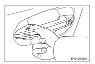
If the door will not lock even when the topside sensor area is touched, try touching both the topside and underside sensor areas at the same time.
