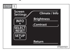
Select "Contrast" on the "Screen Settings" screen, and press the "SELECT RESET" button.
