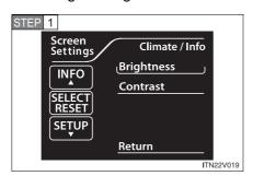
Select "Brightness" on the "Screen Settings" screen, and press the "SELECT RESET" button.
