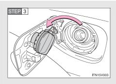
Hang the fuel tank cap on the back of the fuel filler door.
