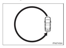
If "C" appears on the display, drive the vehicle at 5 mph (8 km/h) or less in a circle until a direction is displayed.
