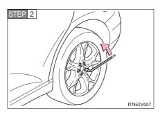
Slightly loosen the wheel nuts (one turn).
