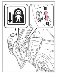
The door cannot be opened from inside the vehicle when the lock is set.
