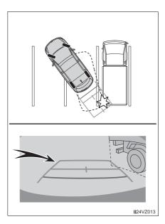
Visually check the surroundings and the area behind the vehicle. In the case shown in the illustration, the truck appears to be outof the vehicle width extension guide lines and the vehicle does not look as if it hits the truck. However, the rear body of the truck may actually cross over the vehicle width extension guide lines. In reality if you back up as guided by the vehicle width extension guide lines, the vehicle may hit the truck.
