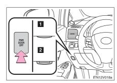
Turn the main switch off to disable the power back door system.
