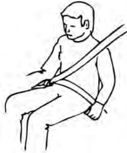
Incorrect (too high on hips)
