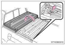
4 Secure by using the storage straps.
