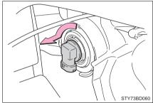
3 Set the new light bulb. Align the 3 tabs on the light bulb with the mounting and insert. Turn it clockwise to set.
