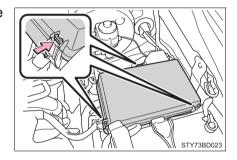
Under the instrument panel Remove the cover.
