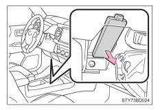
Remove the fuse with the pullout tool.
