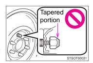
Never use oil or grease on the wheel bolts or wheel nuts. Oil and grease may cause the wheel nuts to be excessively tightened, leading to bolt or disc wheel damage. In addition, the oil or grease can cause the wheel nuts to loosen and the wheel may fall off, causing an accident and resulting in death or serious injury. Remove any oil or grease from the wheel bolts or wheel nuts.
