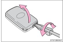
Remove the depleted battery.
