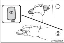
2 Touch the lock sensor (the indentation on the upper part or lower part of the driver's door handle) to lock the doors.
